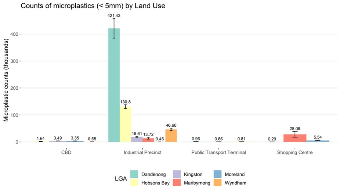
Figure 5: Microplastic data by local government area separated by land use type, including plastic resin pellets, plastic chips/shards from the plastic recycling industry, glass balls used in road marking and polystyrene balls.
