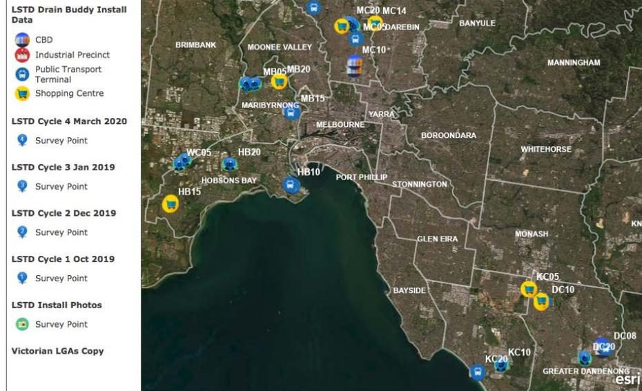
This map illustrates asset locations, installation and servicing cycle data for at-source litter traps used across 6 LGAs in the Let's Strain the Drains Project.
