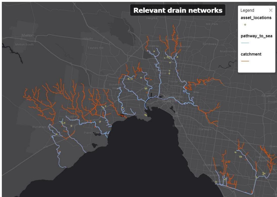
Map 3: This map shows the drainage network that links the stormwater drain locations where traps were installed to Port Phillip Bay.
